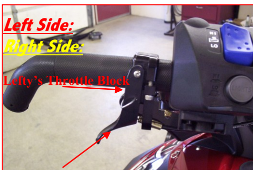
Throttle Lock-Out Pin
